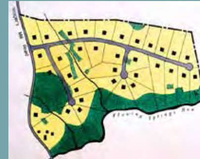
The original site plan called for a conventional subdivision of 34 house lots of 80,000 sq ft (just under 2 acres) each on the 85 acre site, which takes up all the unbuildable land (floodplain, wetland, and steep slopes). Image credits: Randall Arendt, Growing Greener, 1999.
